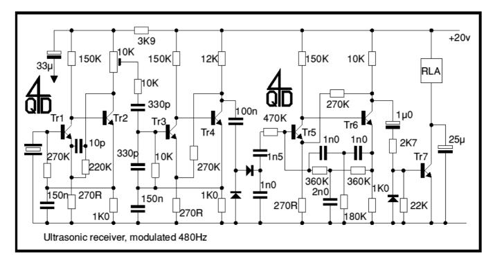
Stage 1 is the preamplifier: it is a fairly conventional circuit with gain fixed by feedback.
