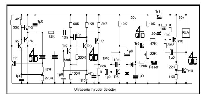
The transmitter circuit is similar to that already shown. Not identical (I think I did this one first - but it was long ago). The preamp (Tr5 & 6) the same as the one in the receiver, but with different values (both work - you can always recalculate values starting with a different initial point and they'll both work).
