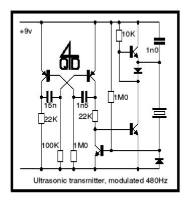
Also, the impedance curve of a piezo device is very complex and I found that some of them resonated at the wrong frequency (too low). A 1n0 cap in series with the resonator cured this - this cap is not shown here.
